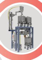
Ensures optimal material quality by blending used and fresh powder for consistent performance
